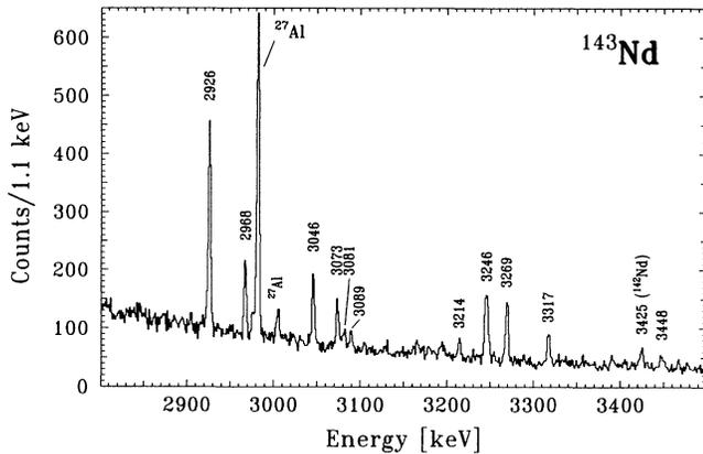
FIG. 1. Spectrum of photons scattered off  $^{143}\text{Nd}$  between 2.8 and 3.5 MeV. The intensive line at 2981 keV arises from a transition in the  $^{27}\text{Al}$  calibration target.
