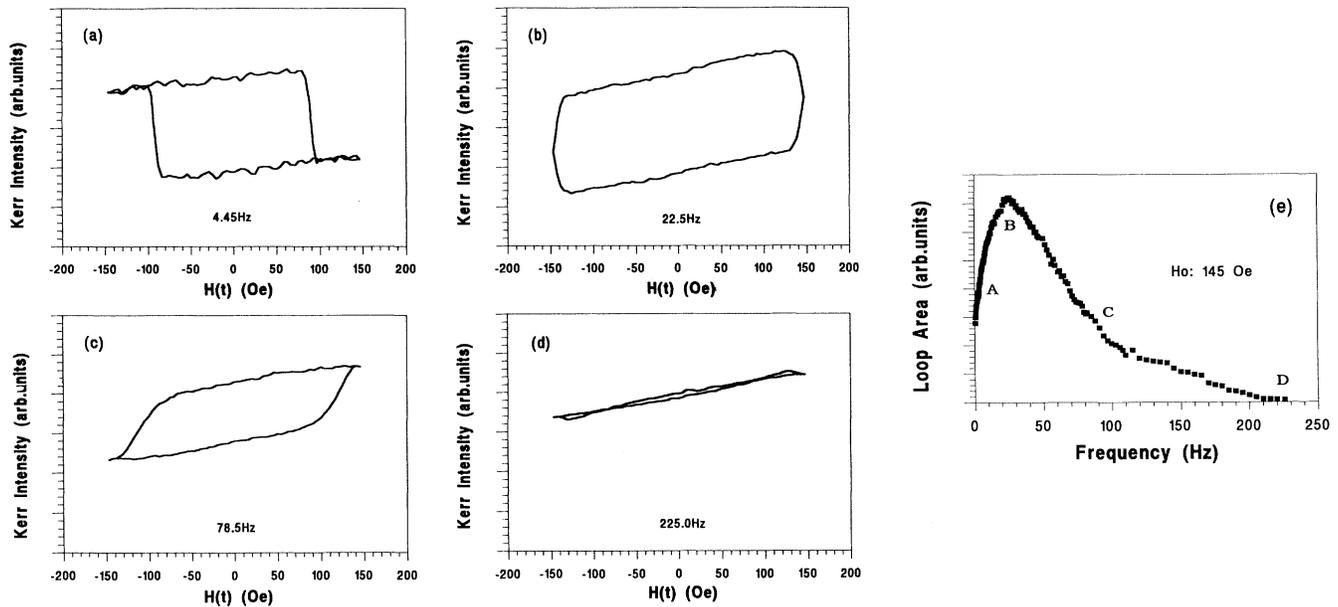
FIG. 1. The hysteresis loops measured at various frequencies: (a) 4.45 Hz; (b) 22.5 Hz; (c) 78.5 Hz; and (d) 225 Hz. The loops are classified as types A, B, C, and D, respectively. (e) The loop area as a function of frequency. The field amplitude was fixed at 145 Oe.
