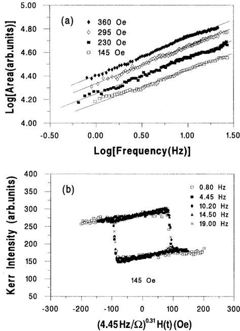
FIG. 2. (a) A log-log plot of the loop area vs frequency at various amplitudes. The slope yields  $\beta=0.31 \pm 0.05$ . (b) The rescaled loops for various frequencies with the amplitude fixed at 145 Oe. The loops are rescaled to the loop of 4.45 Hz according to the power law. The error bar is about the size of the symbol.
