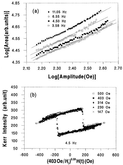
FIG. 3. (a) A log-log plot of the loop area vs amplitude at various frequencies. The slope yields  $\alpha=0.59 \pm 0.07$ . (b) The rescaled loops for various amplitudes with the frequency fixed at 4.5 Hz. The loops are rescaled to the loop of 403 Oe according to the power law. The error bar is about the size of the symbol.
