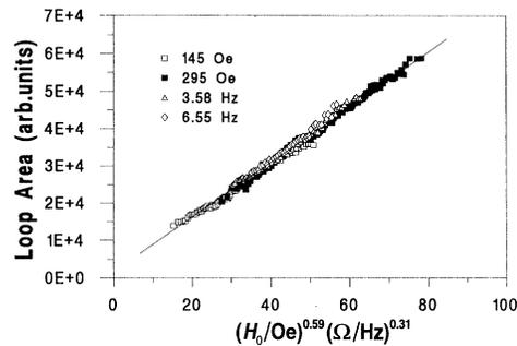
FIG. 4. An area plot which demonstrates the scaling of the hysteresis loops:  $A \propto H_0^{0.59} \Omega^{0.31}$ . The data are taken from Figs. 2(a) and 3(a). The straight line is a guide to the eye.
