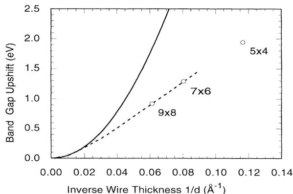
FIG. 2. The band-gap upshift of the wire structures with respect to bulk Si plotted against the inverse of the wire thickness (circles). The EMT upshift of Eq. (2) of the original manuscript with  $C=0.900$  is also plotted (continuous line). The wire thickness  $d$  is defined by Eq. (1) above. The dashed line is an interpolation coinciding with the EMT curve near the origin and passing through the results of the first-principles calculations for the  $9 \times 8$  and  $7 \times 6$  wires.
