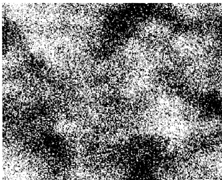
FIG. 5. Simulation for a set of 200 \times 200 lattices with system parameters of Fig. 4 and a diffusion coefficient 10 times smaller. The Z concentration is displayed as gray shades.
