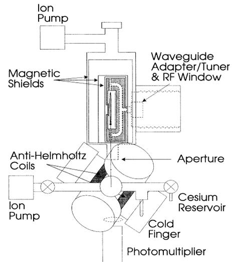
FIG. 1. Fountain schematic. Atoms are trapped in the lower vacuum chamber and launched through the microwave cavity in the upper chamber. Both chambers are pumped by 8 l/s pumps and are separated by a 1.1 cm diam aperture. Microwaves are coupled to the cavity through a coaxial cable connected to the waveguide adapter or tuner and a ceramic vacuum window.
