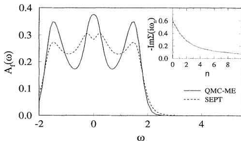
FIG. 1. The  $f$ -electron DOS obtained from QMC and maximum-entropy method (QMC-ME), and that obtained from perturbation theory (SEPT) when  $U=2.0$ ,  $V=0.5$ ,  $\epsilon_d = \epsilon_f = 0$ , and  $T=0.2$ . The corresponding imaginary frequency self-energies are shown in the inset.
