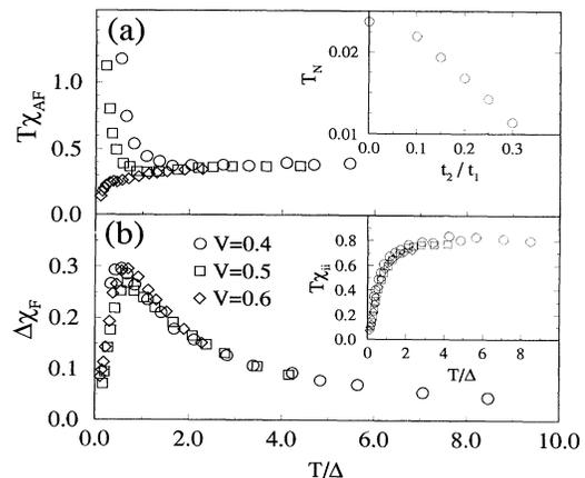
FIG. 5. Susceptibilities of the symmetric PAM when  $U=2.0$  for various values of  $V$ . The inset of (a) shows the Néel temperature  $T_N$  when  $V=0.4$  as a function of a frustrating hopping  $t_2/t_1$ .
