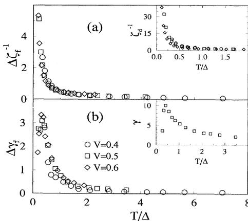
FIG. 4. (a) The  $f$  and  $d$  renormalization factors, and (b) the scaled  $f$  electron  $\gamma_f$  vs  $T/\Delta$  when  $U=2.0$  and  $\epsilon_d = \epsilon_f = 0$ , for various  $V$ . In the inset to (b), the total  $\gamma$  is plotted vs  $T/\Delta$  when  $V=0.5$ .
