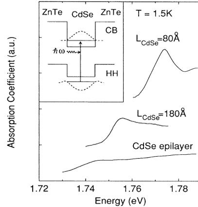
FIG. 2. Absorption spectra of two samples containing single layers of CdSe sandwiched in ZnTe and of a CdSe epilayer are shown on the same scale, indicating the effect of confinement not only in the energies of the transition, but also in the transition probability between the quasibound above-barrier states in the valence band and the bound states in the conduction band (absorption intensity). Inset: The band alignment of the single-barrier heterostructure.
