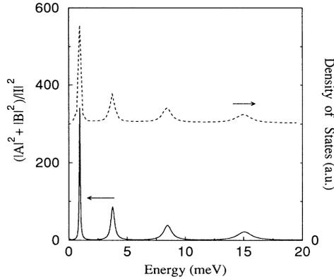
FIG. 1. The ratio of the coefficients  $(|A|^2 + |B|^2)/|I|^2$  (solid line) provides a measure of the localization of the wave function. The dashed line represents the density of states, which peaks at the same energies as the localization. The energy is measured from the top of the barrier.
