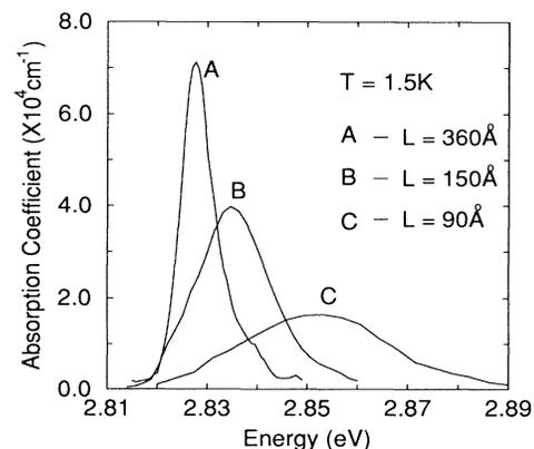
FIG. 3. The absorption coefficients of three single-barrier (ZnMnSe/ZnSe) systems. The clear blueshift of the absorption peak position with decreasing barrier width indicates that the states involved are localized in the barrier.
