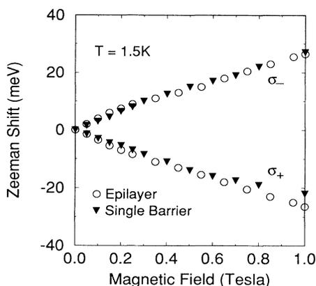
FIG. 4. Experimental results for the Zeeman splittings in the  $\text{Zn}_{0.85}\text{Mn}_{0.15}\text{Se}$  epilayer (circles) and for a 150 Å single barrier (triangles) are plotted as a function of magnetic field. The amount of splitting is very close, indicating that the transition in the single-barrier sample occurs in the  $\text{Zn}_{0.85}\text{Mn}_{0.15}\text{Se}$  barrier layer.
