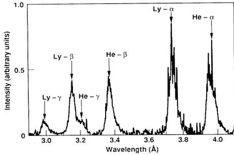
FIG. 2. Measured Ar spectra from an indirectly driven capsule, obtained using the survey spectrometer. Continuum is subtracted and lines are fitted to determine linewidths and intensity ratios.
