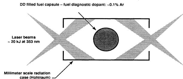
FIG. 1. Schematic diagram of indirectly driven capsule in a hohlraum.
