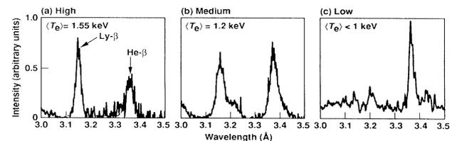
FIG. 5. Measured Ar Ly- $\beta$  and He- $\beta$  lines for (a) “high-” (b) “medium-,” and (c) “low-power” 1-ns drives. Inferred average fuel electron temperatures  $\langle T_e \rangle$  from the RATION code are shown next to the data.
