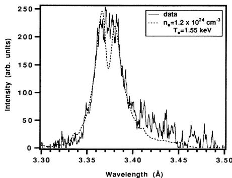
FIG. 4. Measured high-resolution He- $\beta$  line profile for 1-ns “high drive” implosion compared to the calculated line profile at  $n_{e,i} = 1.55 \times 10^{24} \text{ cm}^{-3}$ ,  $T_e = 1.55 \text{ keV}$ . The resolution is 1.5 mÅ.
