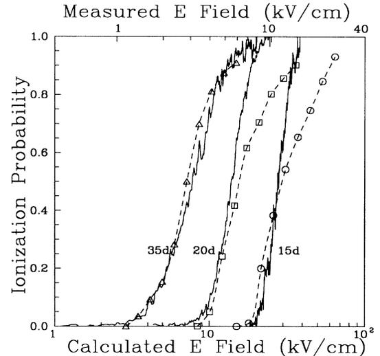
FIG. 3. Measured (solid curves) and calculated (dashed curves) ionization probabilities for the  $30d$ ,  $20d$ , and  $15d$  states as a function of the peak electric field in the HCP. The electric field scales for the numerical and experimental data differ by a factor of 2.5. Note the broad ionization thresholds which are intrinsic to the ionization process.
