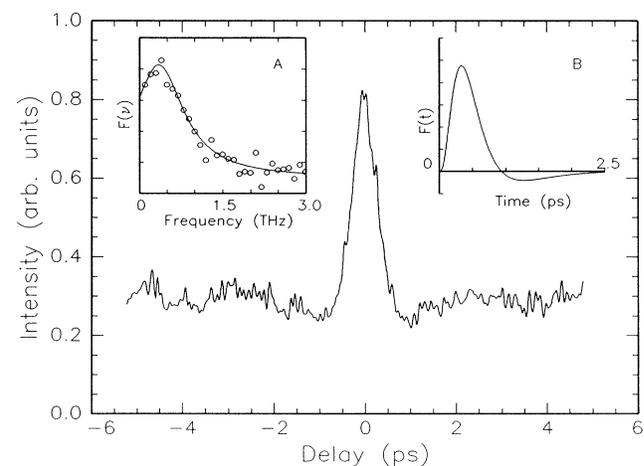
FIG. 1. Electric field autocorrelation as a function of delay in one leg of the Michelson interferometer. Inset (a): Frequency spectrum of the HCP. Inset (b): Inferred temporal pulse shape of the HCP.
