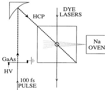
FIG. 2. Schematic diagram of the interaction region shown from above. The HCP is produced by applying a 100 fs laser pulse to the GaAs wafer which shorts the high voltage (HV) across the photoconducting surface. The transmitted radiation is weakly focused with a parabolic mirror. The two pulsed dye lasers and the HCP interact with the Na beam between two parallel conducting plates.
