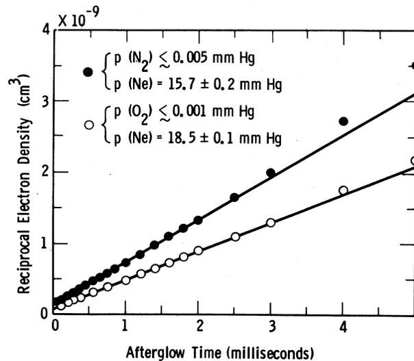
FIG. 2. Time variation of the reciprocal electron density in the afterglow of high-pressure  $\text{N}_2$ -Ne and  $\text{O}_2$ -Ne microwave discharges.
