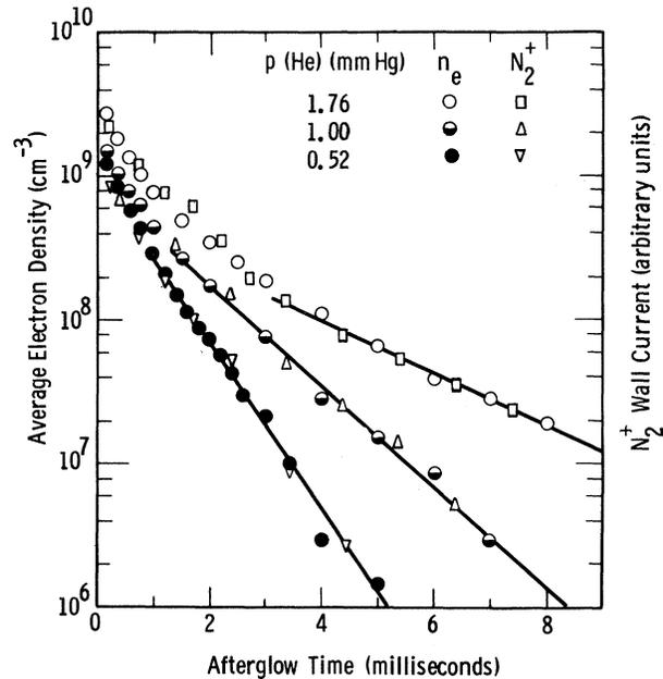
FIG. 1. Electron and N<sub>2</sub><sup>+</sup> ion decay in the afterglow of N<sub>2</sub>-He microwave discharges having constant nitrogen pressure, 0.006 mm Hg, and variable helium pressure. The N<sub>2</sub><sup>+</sup> wall currents are normalized to the respective electron density decay curves at an afterglow time of approximately 2 milliseconds.
