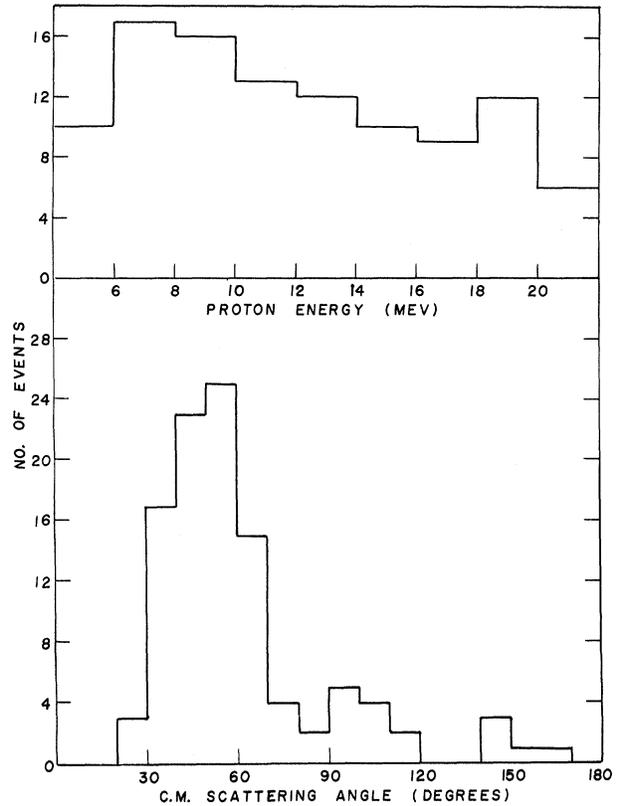
FIG. 2. (a) Proton energy spectrum of Sample A ( $\theta \geq 26^\circ$ ,  $4 \text{ Mev} \leq \epsilon \leq 22.5 \text{ Mev}$ ). (b) Center-of-mass angular distribution of Sample A.
