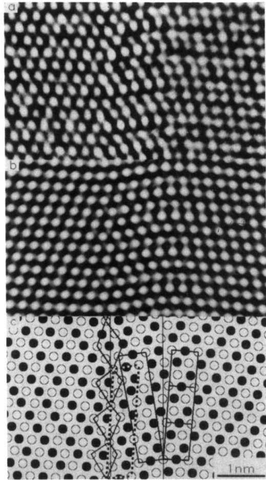
FIG. 2. The (a) observed and (b) simulated HRTEM images of the grain boundary in Ag. (c) The atomic coordinates (x,y) extracted from (a) and used for the simulation (b). The black and white shading is our assignment of atoms to one of the two (220) planes in the z direction.
