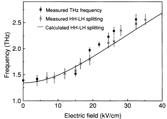
FIG. 4. Measured THz frequencies, lh-hh splittings taken from photocurrent spectra, and calculated lh-hh splittings as a function of electric field in the MQW. The calculation includes excitonic effects.
