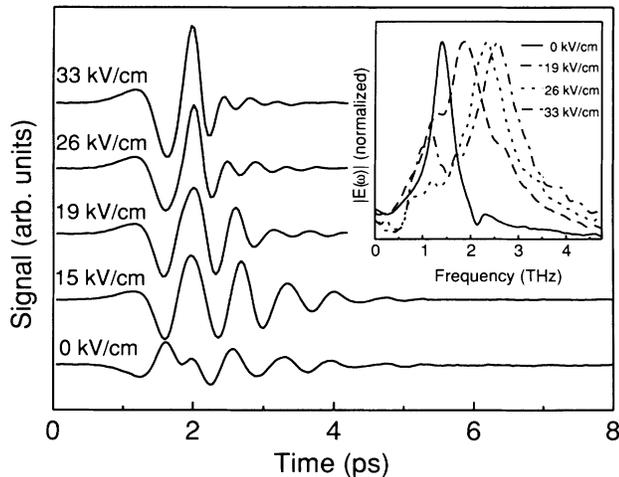
FIG. 3. Measured THz wave forms for several electric fields in the MQW. The laser is tuned to the lh and hh excitons. Inset: The Fourier transforms of only the oscillatory part of the signals.
