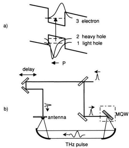
FIG. 1. (a) Wave-function envelopes of the electron, lh, and hh in a quantum well biased with an electric field  $E$ . (b) Experimental setup for the THz generation measurements with multiple quantum well (MQW).
