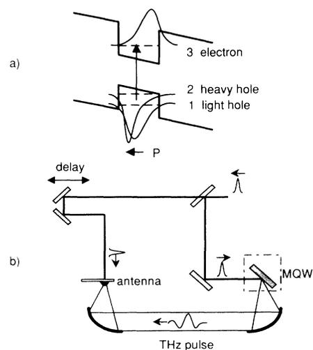
FIG. 1. (a) Wave-function envelopes of the electron, lh, and hh in a quantum well biased with an electric field  $E$ . (b) Experimental setup for the THz generation measurements with multiple quantum well (MQW).
