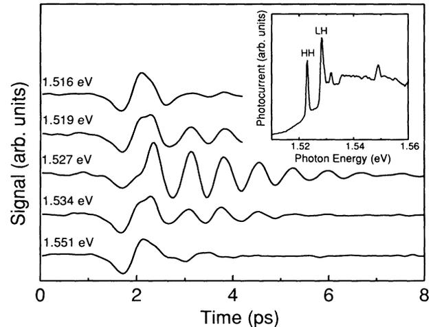
FIG. 2. Measured THz wave forms for several excitation wavelengths. The electric field in the MQW is 4 kV/cm. Inset: The measured photocurrent spectrum.
