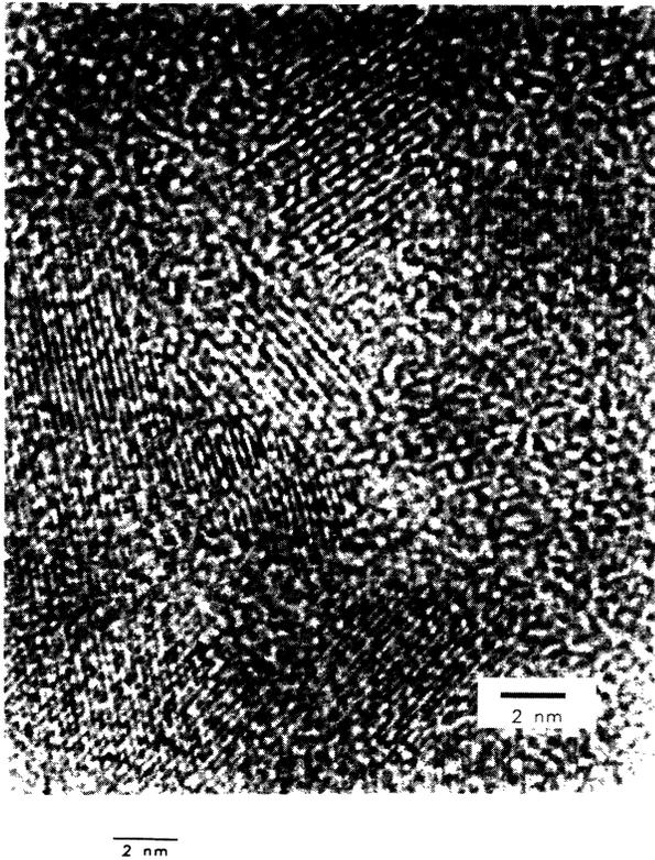
FIG. 1. High-resolution electron micrograph of  $\alpha$ -quartz after pressurization to 20.0 GPa.
