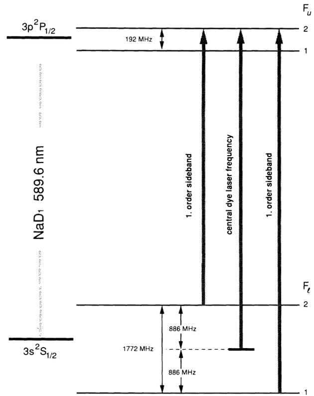
FIG. 2. Energy levels corresponding to the  $D_1$  line of Na. Thick grey arrows indicate pump laser frequency and the two first-order sidebands produced by the electro-optical modulator (cf. text).
