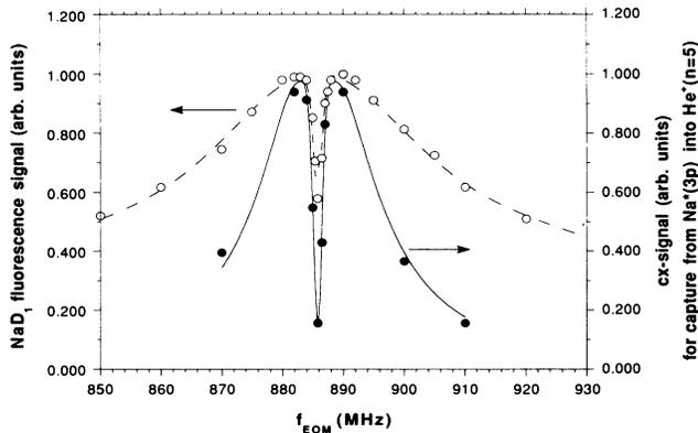
FIG. 3. Intensity of Na  $D_1$  fluorescence and cx signals for capture into  $\text{He}^+(n=5)$  from excited  $\text{Na}^*(3p)$  as a function of the microwave frequency applied to the electro-optical modulator. The cx signal is proportional to the number of excited  $\text{Na}^*(3p)$  atoms as seen by the probing ion beam.
