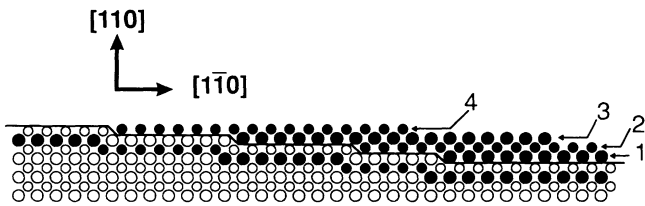
FIG. 4. Schematic diagram of "intermixed Stranski-Krastanov" growth mode for Au/Ag(110). Solid (open) circles indicate Au (Ag) atoms. Two circle sizes denote atoms in different vertical (001) planes. Line shows step positions after intermixed layer is complete but before fingers grow. For clarity, steps are drawn more closely spaced than in actual sample.
