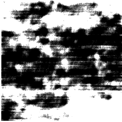
FIG. 6. An image, 15 nm on a side, taken at the large sample bias of +1 V, with 50-pA average current. Note the large, 1–2-nm swells and depressions; these bear no simple geometrical relation to the atomic structure measured at smaller bias values, and may be related to the electronic effects of oxygen disorder.
