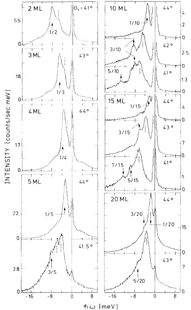
FIG. 1. Inelastic He-atom energy transfer spectra of Na ultrathin films on Cu(001) for  $N_L=2$  to 20 monolayers (ML) along a  $\langle 100 \rangle$  direction of the substrate. Each fraction  $(2n-1)/N_L$  labels the  $n$ th organ-pipe mode. The Rayleigh modes of the substrate (broken bar) and of the film (solid bar) are also indicated.
