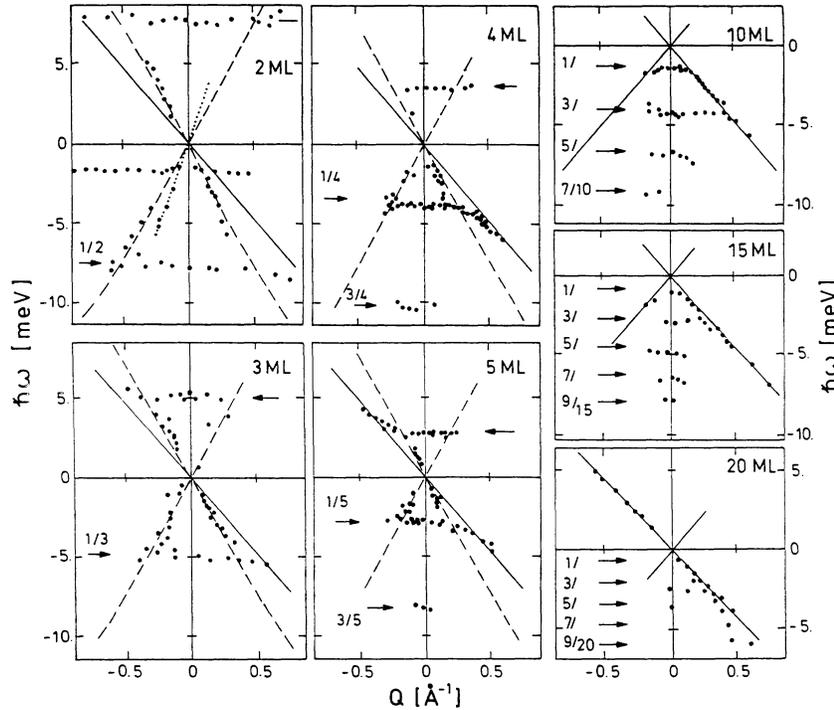
FIG. 2. Measured dispersion curves of Na films (2 to 20 ML) on Cu(001). The arrows indicate the theoretical positions of the organ-pipe modes. The directions of the Rayleigh wave branches in the film (solid line) and in the substrate (broken line) are also shown. For 2 ML a few points correspond to the longitudinal resonance of the substrate (dotted line).
