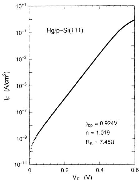
FIG. 1. Forward  $I$ - $V$  characteristic at 295 K of a Hg/Si(111) Schottky diode with a diameter of 1000  $\mu\text{m}$  representing a barrier height of 0.924 V and an ideality factor of 1.019. The silicon surface was etched for 30 s in 10:1 diluted HF and rinsed for 30 s in deionized water.
