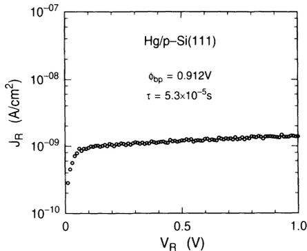
FIG. 2. Reverse  $I$ - $V$  characteristic at 295 K of a Hg/Si(111) Schottky diode with a diameter of  $1000\ \mu\text{m}$  representing a barrier height of  $0.912\ \text{V}$  and a carrier lifetime of  $5.3 \times 10^{-5}\ \text{s}$ . The silicon surface was etched for 30 s in 10:1 dilute HF and rinsed for 30 s in deionized water.
