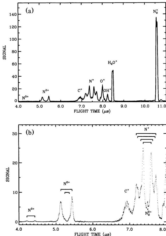
FIG. 2. An average (2688 laser pulses) 193-nm, 12-ps  $N_2$  spectrum with the background (an average of 512 laser pulses) subtracted. Each spectrum was obtained with a temporal resolution of 1 ns and with power densities ranging from  $10^{14}$  to  $10^{15}$  W/cm<sup>2</sup>. The doublet in the  $N_2^{2+}$  peak is an artifact of an incomplete subtraction due to saturation of the scope.
