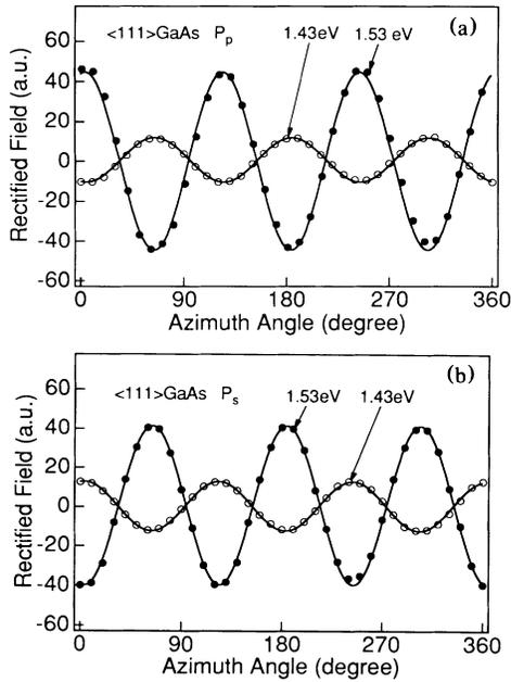
FIG. 3. Rectified field vs azimuth angle at two optical polarizations (a) parallel and (b) perpendicular to the detector axis. The open and solid circles are the experimental data at two photon energies (1.43 and 1.53 eV, respectively). The curves are plots of the rectified field calculated from the nonlinear polarizations (a)  $P_p$  and (b)  $P_s$  (the sign is reversed).
