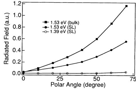
FIG. 4. Rectification signal vs optical incident angle (polar angle) from a  $\langle 111 \rangle$ -oriented GaAs bulk and GaAs/ $\text{In}_{0.1}\text{Ga}_{0.9}\text{As}$  superlattice at three photon energies.
