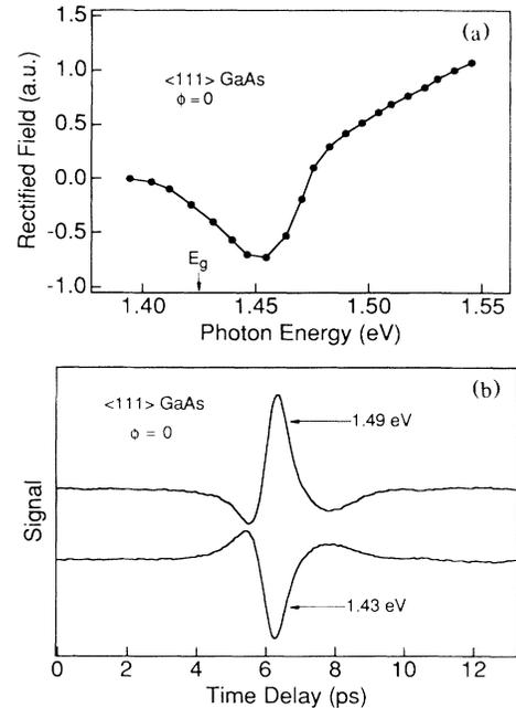
FIG. 2. (a) The peak value of the rectified signal vs laser energy at normal optical incident angle, from  $\langle 111 \rangle$  GaAs. (b) Temporal wave forms of the radiated field at a photon energy of 1.49 eV (upper trace) and 1.43 eV (lower trace), respectively.
