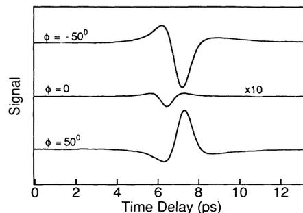
FIG. 1. THz radiation from a  $\langle 111 \rangle$ -oriented GaAs with normal (center trace) and  $\pm 50^\circ$  (lower and upper traces) optical incident angles. Temporal broadening of the THz radiation wave form is pronounced with the oblique optical beams.
