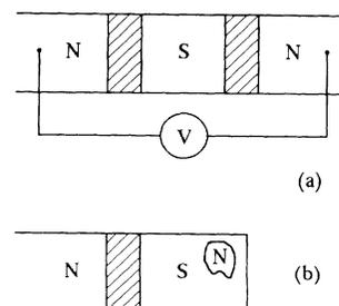
FIG. 1. The two systems under consideration: (a) ideal superconducting electrode between normal bulk electrodes forming two tunnel junctions in series; (b) superconducting "single-electron box" with small normal inclusion. Dashed regions denote tunnel barriers.
