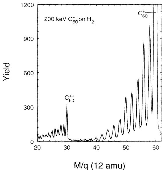
FIG. 1.  $M/q$  (mass divided by charge) spectrum resulting from fragmentation of 200-keV  $C_{60}^+$  colliding with  $H_2$ . The right- and left-hand parts reflect singly and doubly charged fragments, respectively.
