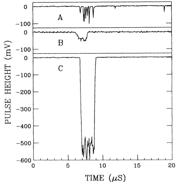
FIG. 2. Curve *A*: The wave form of the *best* slow-particle candidate. *B*: The wave form of an LED-simulated event having the same signal charge as *A*. *C*: A simulated wave form of a nuclearite with this pulse width ( $\beta=3 \times 10^{-4}$ ). All the wave forms are drawn to the same scale.
