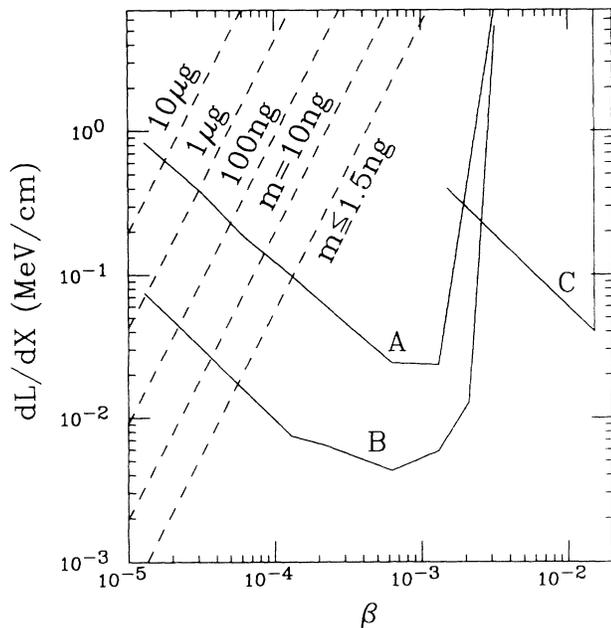
FIG. 1. Light yield of nuclearites in the MACRO scintillator as a function of velocity ( $\beta=v/c$ ) for different masses of nuclearites (dashes). The solid curves are the 90%-trigger efficiency contours of the MACRO slow-particle trigger system. Curve *A*: Type-I trigger based on time of passage in one scintillator counter before summer 1989. *B*: The same type-I trigger after summer 1989. *C*: Type-II trigger based on the time of flight between scintillator counters.
