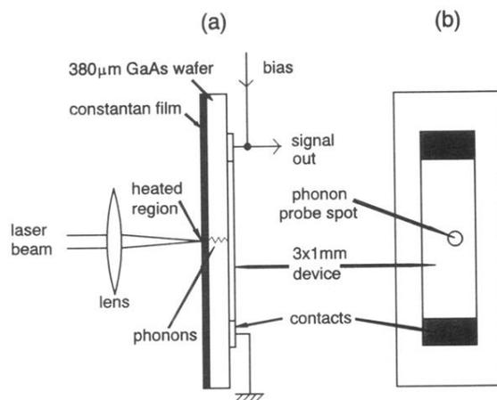
FIG. 2. Sample geometry: (a) Side view, the laser beam is positioned on the Constantan film using a pair of galvanometer driven  $x$ - $y$  mirrors under computer control. (b) Top view (sample face), the light-shaded area indicates the approximate size of the phonon probe beam.
