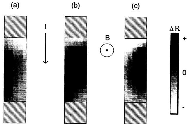
FIG. 4. Images of the change in two-terminal resistance at three different filling factors. (a)  $E_F$  just below an empty Landau level, (b)  $E_F$  midway between two levels, and (c)  $E_F$  just above a filled level.
