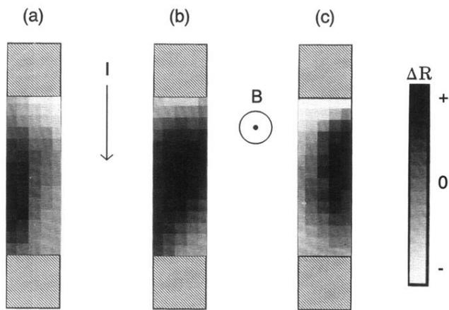
FIG. 4. Images of the change in two-terminal resistance at three different filling factors. (a)  $E_F$  just below an empty Landau level, (b)  $E_F$  midway between two levels, and (c)  $E_F$  just above a filled level.
