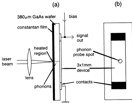
FIG. 2. Sample geometry: (a) Side view, the laser beam is positioned on the Constantan film using a pair of galvanometer driven  $x$ - $y$  mirrors under computer control. (b) Top view (sample face), the light-shaded area indicates the approximate size of the phonon probe beam.
