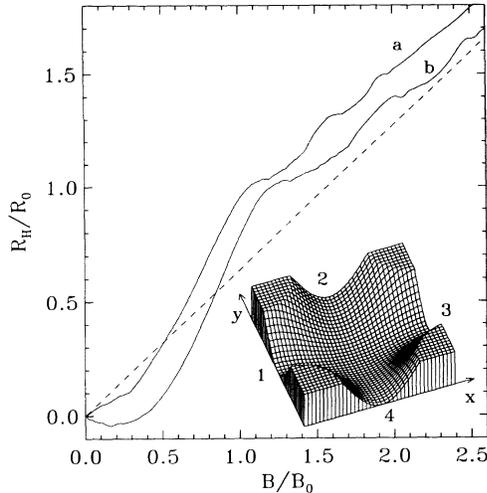
FIG. 1. Hall resistance  $R_H$  vs magnetic field for a smooth model potential of a cross junction (inset with lead numbers) with  $\hat{r} = 1/2$  and  $\hat{f} = -1/3$  (curve a) showing the last Hall plateau and two additional plateaus. For  $\hat{f} = -1$  (curve b) the additional plateaus are shifted to higher values of  $R_H$  and still lie above the 2D Hall resistance of free electrons (dashed line). The latter is approached asymptotically for higher magnetic fields.
