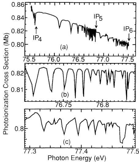
FIG. 1. Photoionization spectrum of He  $1P^\circ$  states: (a) below the  $N = 5$  and  $6$  thresholds ( $IP_5$ ,  $IP_6$ ), (b) magnification of the high- $n$  region below the  $N = 5$  threshold, (c) magnification of the high- $n$  region below the  $N = 6$  threshold.
