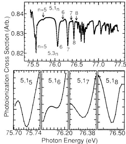
FIG. 2. Photoionization spectrum of He convoluted with experimental resolution of 6 meV below the  $N = 5$  and  $6$  thresholds. Resonances labeled  $5, 1_n$  are magnified underneath. Note that the dots are calculated points and the solid lines simply join them smoothly.
