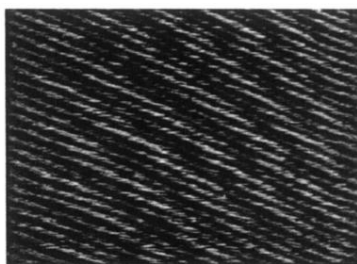
FIG. 4. STM image of a C_{192}H_{386} monolayer at the interface between an organic solution and graphite, imaged at 65^\circ\text{C} . The slight modulation in contrast, perpendicular to the main molecular axes, may be attributed to a finite angle with the carbon chain axis in the underlying graphite lattice (see also [11,13]).
