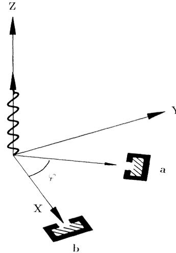
FIG. 1. Coordinate frame and experimental setup. Circularly polarized light is incident along the  $z$  direction. One electron counter ( $b$ ) is in the  $x$  direction whereas the other one ( $a$ ) can be rotated in the  $x$ - $y$  plane.
