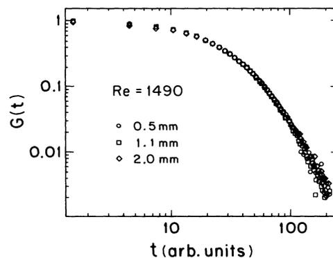
FIG. 1. Superimposed log-log plot of  $G(t)$  for the three indicated slit widths  $L$  and at the Reynolds number indicated.
