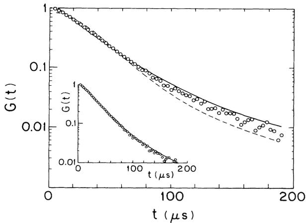
FIG. 2. Semilog plot of  $G(t)$  at  $Re=1490, L=1.3$  mm. The solid line is a Lorentzian fit to the data, and the dashed line is a Gaussian fit. The characteristic widths  $u_L(L)$  and  $u_G(L)$  of both factors are 0.216 cm/sec. The inset shows the same data fitted using Eqs. (1) and (2).
