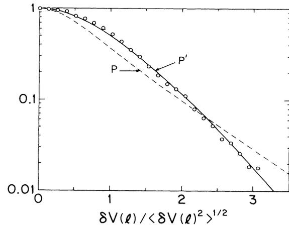
FIG. 3. Semilog plot of the symmetric part of the probability density function as measured by laser Doppler velocimetry, the abscissa being  $\delta v(l)/[\langle \delta v(l)^2 \rangle]^{1/2}$ . The solid line is a fit to these data using Eq. (1) and the dashed line is the function  $P$  extracted from the HCS measurements, using Eqs. (1) and (2). The measurements were at  $Re=1490$  and  $L=1.3$  mm.
