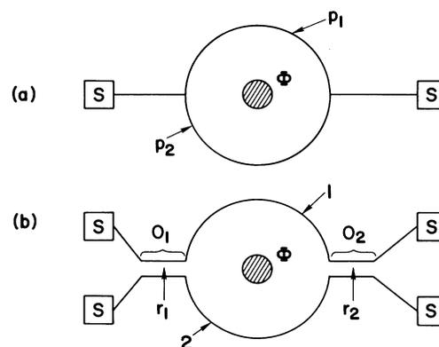
FIG. 1. (a) Direct interference: Wave transmitted from source ( $S$ ) to sink ( $S$ ) is split into partial waves encircling the flux. (b) Exchange interference: Two waves transmitted from sources to sinks without encircling the flux but with an overlap in regions  $O_1$  and  $O_2$ .
