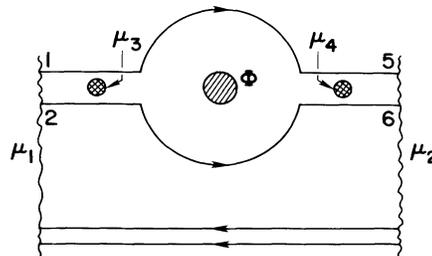
FIG. 2. Conductor with two edge states at the upper boundary coupling with interior contacts 3 and 4.
