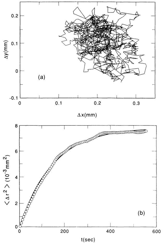
FIG. 3. (a) The trajectory of a defect over a 2-h time period at 74.6 °C. (b) Mean-square displacement vs time for the data in (a). The saturation of  $\langle \Delta r^2 \rangle$  at long times shows the effect of the binding potential on the motion.
