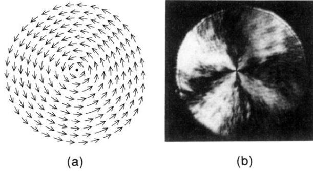
FIG. 1. (a) The topological defect studied in these experiments: a  $2\pi$  ( $s = +1$ ) point bend disclination in  $\mathbf{c}(\mathbf{r})$ , the 2D nematic director field of a freely suspended smectic-C film. (b) Appearance of the vortex of (a) in depolarized reflected light microscopy (DRLM) [9]. The diameter of the illuminated area is 1.8 mm. The film diameter is 3.7 mm.
