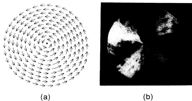
FIG. 1. (a) The topological defect studied in these experiments: a  $2\pi$  ( $s=+1$ ) point bend disclination in  $\mathbf{c}(\mathbf{r})$ , the 2D nematic director field of a freely suspended smectic-C film. (b) Appearance of the vortex of (a) in depolarized reflected light microscopy (DRLM) [9]. The diameter of the illuminated area is 1.8 mm. The film diameter is 3.7 mm.
