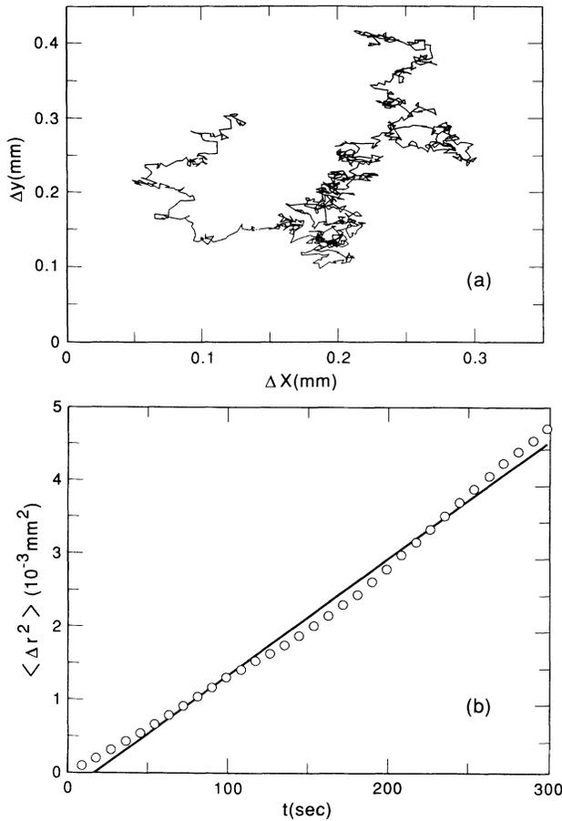
FIG. 2. (a) The trajectory of a defect over a 2-h time period at 55.1 °C. (b) Mean-square displacement vs time for the data in (a), giving a diffusion constant  $D=0.8 \times 10^{-7} \text{ cm}^2/\text{sec}$ .
