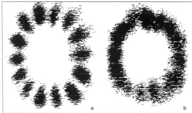
FIG. 3. Spatial intensity distribution of the laser: (a) At low excitation current 14 maxima with the same radial coordinate and equally spaced in the azimuthal direction are observed. (b) At high excitation current a ring appears superimposed to the SW. The intensity is time independent evidencing that the SW and TW superimposed have the same frequency.
