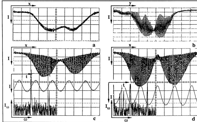
FIG. 5. Intensity across different patterns in a laser with the central region active. (a) Standing wave solution. (b),(c) Cylindrically symmetric+(SW+TW) solution. (d) Cross section of a MW solution. Two frequencies are observed in the power spectrum.
