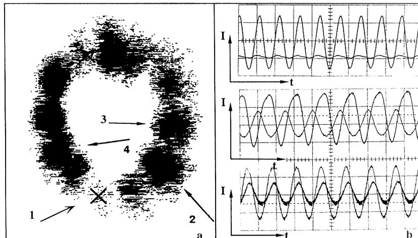
FIG. 4. (a) Intensity distribution during transients. (b) From top to bottom: Transient oscillations of the intensity. The high amplitude signal was taken in point 3 of (a). The low amplitude signal corresponds to points 1 (source of waves), 2, and 4 of (a), respectively.
