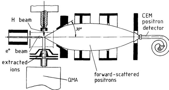
FIG. 1. The layout of the hydrogen scattering experiment: The ion rate of the quadrupole mass analyzer (QMA) is measured. In addition, the ion detector of the QMA provides the "start pulse" for the time-correlation measurement, while the time-delayed positron-detection signal from the channel electron multiplier (CEM) provides the "stop pulse."
