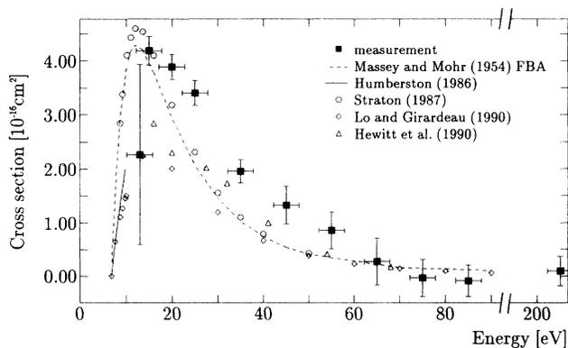
FIG. 2. Measured Ps-formation cross sections (solid squares with error bars); the vertical bar represents the statistical error of the data point, and the horizontal bar, the energy uncertainty. Also plotted are several theoretical predictions explained in the text.
