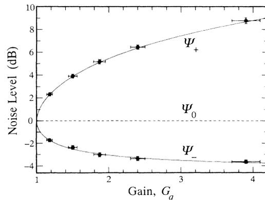
FIG. 2. Logarithm of observed noise levels  $\Psi_+$  (maximum) and  $\Psi_-$  (minimum) vs OPO gain  $G_q$  for a squeezed beam at balanced detector 1 (cf. Fig. 1).  $\Psi_0$  is the vacuum-state level and  $\Omega/2\pi = 1.1$  MHz for these data. The solid curves are theoretical fits as discussed in the text.
