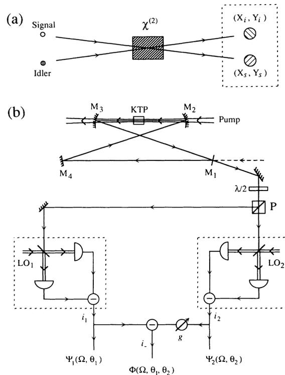
FIG. 1. (a) Scheme for realization of the EPR paradox by nondegenerate parametric amplification, with the optical amplitudes ( $X_s, Y_s$ ) inferred in turn from ( $X_i, Y_i$ ). (b) Principal components of the experiment.
