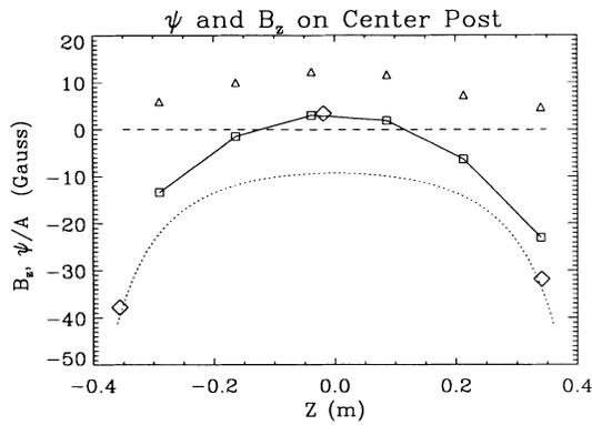
FIG. 4. Measurements on the center post of the device ( $R=8$  cm).  $\square$ , total  $B_z$  (plasma and external coil current) showing field reversal;  $\triangle$ ,  $B_z$  of plasma current;  $\diamond$ , total flux ( $\psi_{vac} + \psi_{plasma}$ ); and the dotted line,  $\psi_{vac}$ .
