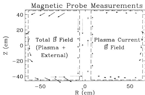
FIG. 3.  $B_p$  field as measured on vacuum vessel wall. The right half is the field due to  $I_{plasma}$  and the left the total field which includes the field from external coil. Measurement on the top, bottom, and outside walls are by 2D pickup loops ( $B_r$  and  $B_z$ ), and the inner wall measurements are  $\psi$  and  $B_z$  loops. The origin of each vector indicates the probe position.
