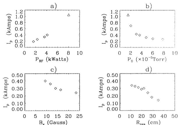
FIG. 2. Parameter scan showing phenomenological dependencies of open field line currents:  $I$  vs (a) ECR power, (b) neutral pressure, (c) mirror field strength, in terms  $B_z$  at  $Z = 0$  cm,  $R = 30$  cm, (d) ECRH resonance radius (i.e.,  $B_\theta$ ). Unless varied, values are 4 kW,  $P_0 = 3 \times 10^{-5}$  Torr,  $B_z = 10$  G,  $R_{ECH} = 10$  cm. The 1.05-kA point ( $\Delta$  shown for reference), was at 8 kW,  $P_0 = 1 \times 10^{-5}$  Torr.
