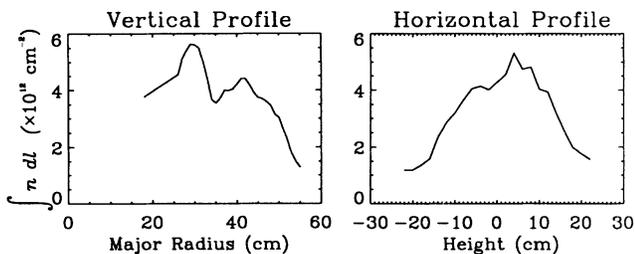
FIG. 5. Line integral density profiles as provided by a 2D interferometry system.
