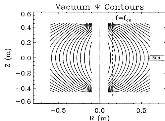
FIG. 1. The vacuum poloidal flux contours. The total field is a combination of  $\nabla\psi \times \nabla\phi$  ( $\psi$  being the poloidal flux function) and a toroidal field  $B_\phi = B_0 R_0/R$ .
