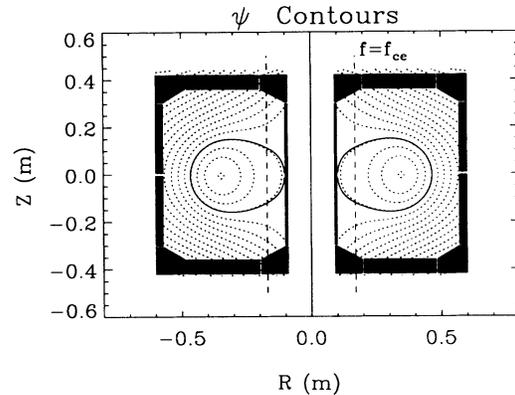
FIG. 6.  $\psi$  contours as modeled by filament currents matched to the boundary magnetic field measured by magnetic pickup and flux loops. Also shown is the isolated limiter array defining the outermost closed flux surface and measuring currents flowing from the plasma to the vessel.
