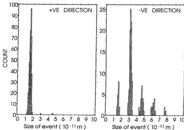
FIG. 2. Distribution of sizes of phase slip events for orifice 1, in terms of the associated amplitude loss from the resonator. Separate histograms are shown for the two flow directions.  $T = 0.27$  K.
