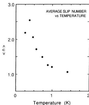
FIG. 3. The variation of the average slip number  $\langle n \rangle$  with temperature for the direction exhibiting multiple slips in orifice 1. At a given temperature, the average is taken over all the events in that flow direction. Above 1.5 K it is not possible to resolve individual phase slips due to the low  $Q$  of the resonator. However, the critical velocity  $v_c$  can still be identified from a plot of oscillator amplitude vs applied drive.
