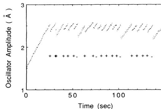
FIG. 1. Phase slips in the time evolution of resonator amplitude at  $T=0.26$  K for orifice 1. Resonator  $Q$  is  $\sim 10^4$ . The plus or minus sign shown below each jump gives the direction of flow through the orifice at the time of the phase slip.
