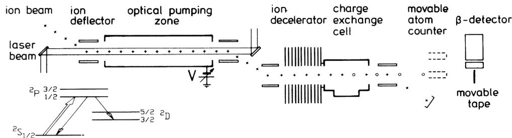
FIG. 1. Experimental setup. Inset: The low-energy electronic level scheme of Ca II and the laser optical pumping cycle are shown.
