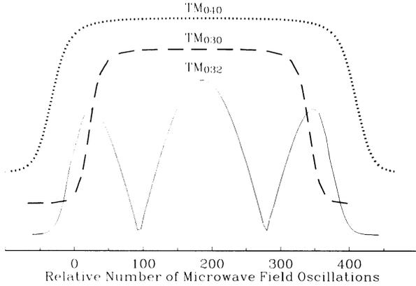
FIG. 1. Absolute value  $|A(t)|$  of the experimental pulse shape, displaced vertically for clarity, for each of three microwave frequencies: Top, 36.02 GHz; middle, 26.43 GHz; bottom, 30.36 GHz.
