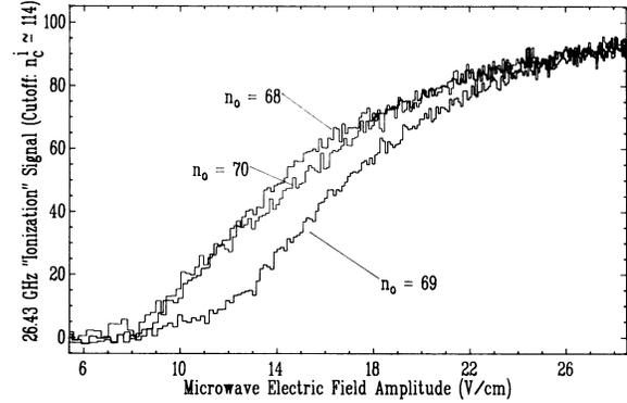
FIG. 2. Measured “ionization” curves for  $n_0=68,69,70$  3d H atoms in a 26.43-GHz field, with the middle pulse shape shown in Fig. 1.
