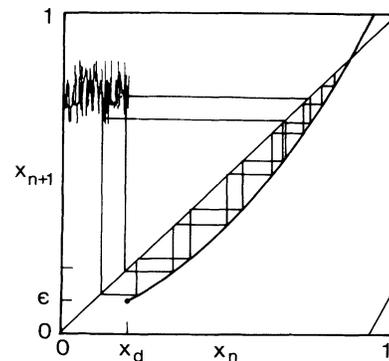
FIG. 1. The considered mapping  $x_{n+1} = f(x_n)$  with a point of discontinuity at  $x_d = 2\epsilon$  and the parameters  $\epsilon = 0.1$ ,  $s = 0.5$ . Additionally, the path of one iteration is shown; the iteration is reinjected stochastically into the laminar region after passing  $x_d$ .
