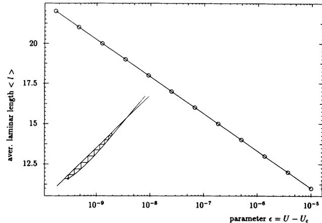
FIG. 3. Results for the thyatron relaxation oscillator. Average laminar length  $\langle l \rangle$  for different values of the control parameter. Again the result of (4) can be confirmed. Inset: A part of the multimap  $f^{12}(x)$  vs  $x$ , showing a situation quite similar to the constructed mapping in Fig. 1.
