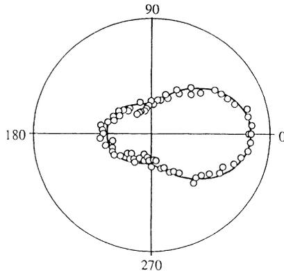
FIG. 1. Polar plots of the square root of the SHG signal as a function of the angle between the surface rubbing direction and the plane of incidence. Both the input and output beams are  $p$  polarized. The circles are experimental data; the solid line is the theoretical fit.
