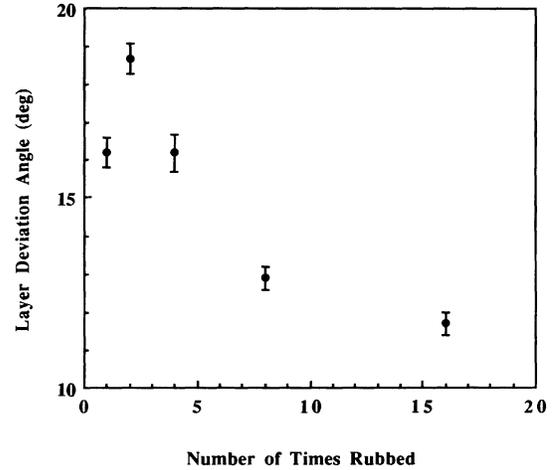
FIG. 3. The layer deviation angle as a function of the number of times the substrate was rubbed. The homogeneity of the sample alignment was rather poor for the substrate that was rubbed only once. Thus the trend of larger deviation angles for weaker rubbing is finally limited by a deterioration of the monodomain alignment for very weak rubbing.
