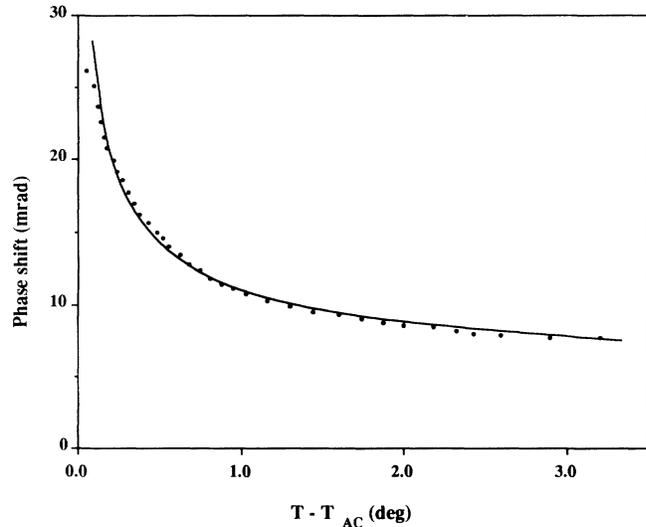
FIG. 2. The phase shift as a function of temperature. The circles are the experimental data; the solid line is a fit by the theory.
