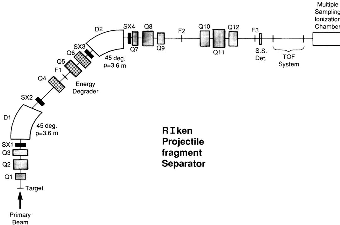
FIG. 1. Schematic drawing of the facility at RIKEN used to produce the  ${}^8\text{Li}$  beam and study the  ${}^4\text{He}({}^8\text{Li}, {}^{11}\text{B})n$  reaction. The various elements are denoted by the symbols  $D_j$  (dipole magnet),  $F_j$  (focus point),  $Q_j$  (magnetic quadrupole), or  $SX_j$  (magnetic sextupole).
