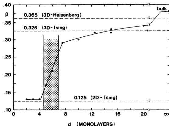
FIG. 2. Critical exponent  $\beta$  as a function of film thickness (error bars are given in Table I). The dashed lines show the theoretical values for a 3D Heisenberg, 3D Ising, and 2D Ising system. The shaded regime marks the crossover from 3D to 2D.
