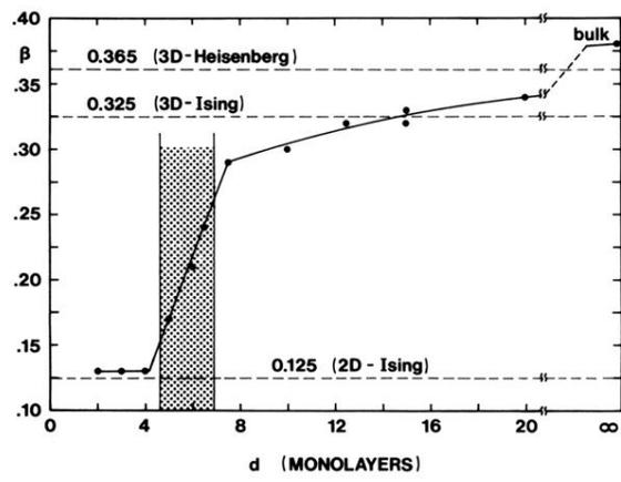
FIG. 2. Critical exponent  $\beta$  as a function of film thickness (error bars are given in Table I). The dashed lines show the theoretical values for a 3D Heisenberg, 3D Ising, and 2D Ising system. The shaded regime marks the crossover from 3D to 2D.
