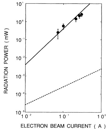
FIG. 3. The measured power (dots) of the spontaneous emission as a function of the electron-beam current. The dashed and solid lines represent the theoretically calculated power of incoherent and coherent radiation, respectively. The coherent radiation power is theoretically calculated for radiation with a wavelength of 7.4 mm and an electron-beam pulse width of 33 ps. The number of electrons in a micropulse is estimated to be  $5 \times 10^8$  for a 0.5-A RPE current.
