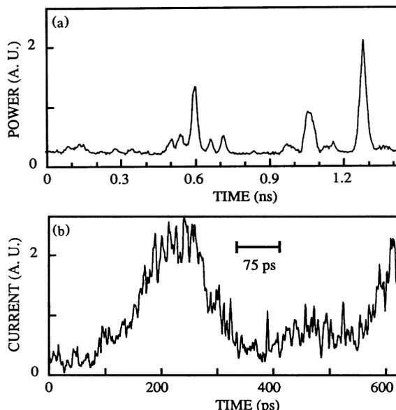
FIG. 2. (a) Typical wave form of the fourth harmonic of a Q-switched Nd-YAIG laser, which was measured using a streak camera using 12-ps temporal resolution. (b) Typical wave form of the electron-beam micropulse. The marker of 75 ps represents the value of the pulse width broadened by the dispersion of the Cherenkov radiation and multimode quartz fiber.
