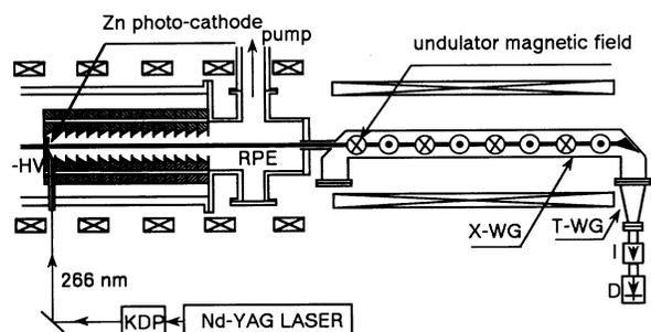
FIG. 1. Schematic diagram of spontaneous emission experimental setup (RPE denotes relativistic photoelectron beam, D denotes 1N26C microwave diode, I denotes isolator, X-WG denotes X-band waveguide, and T-WG denotes tapered waveguide).
