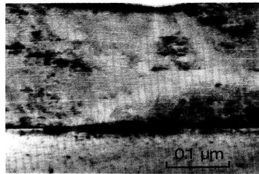
FIG. 1. Cross-section transmission electron micrograph of a  $1 \times 8$  YBCO/PBCO superlattice. The 11.7-Å lattice fringes clearly indicate undulations in the layers.
