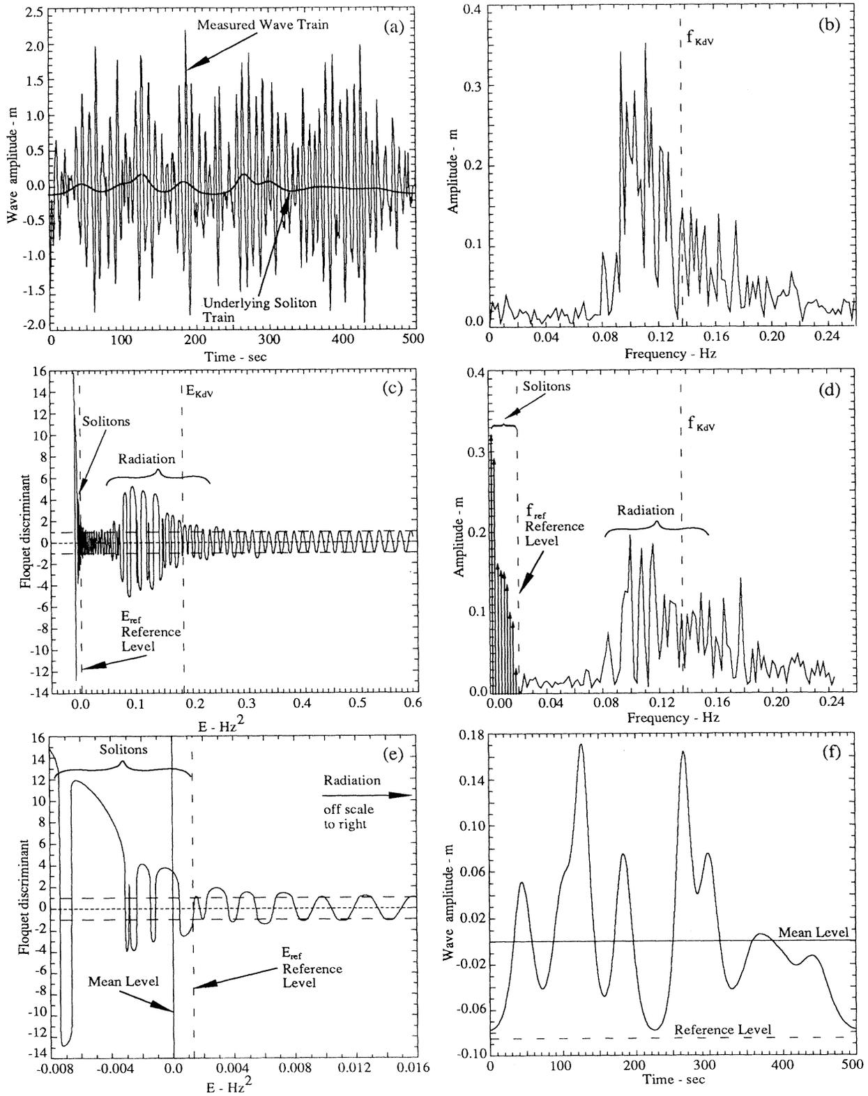
FIG. 1. (a) Measured times series with  $H_s=3.0$  m,  $T_d=9.1$  sec, and  $h=16.5$  m. (b) Fourier spectrum of (a). (c) Floquet discriminant of (a); the soliton and radiation parts of spectrum are well separated. (d) Scattering transform of (a). (e) Floquet discriminant in the *soliton part* of the spectrum of (a). (f) Soliton train obtained by filtering out the radiation spectrum and inverting the scattering transform of (d); solitons are also graphed in (a) at the same scale as the data.
