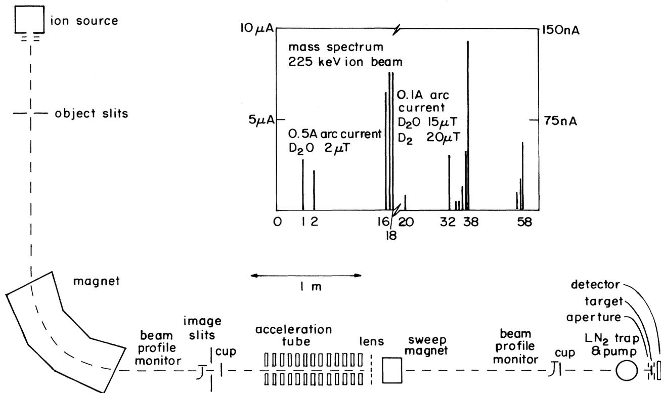
FIG. 1. Diagram of experimental apparatus. Inset: Two mass spectra. The left part of the inset shows the low mass spectrum when there was still appreciable residual  $^1\text{H}$ , and the right part shows the mass spectrum after optimization of  $n=2$  and 3 clusters by addition of  $\text{D}_2$  gas.
