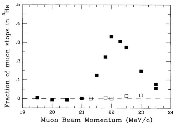
FIG. 2. The fraction of muons stopped in the  $^3\text{He}$  as a function of beam momentum. The open squares represent a thick-walled target in which all muons stopped in the glass. The solid squares represent a standard target cell. The data points at 23.5 MeV/c were taken at muon rates differing by a factor of 2. The statistical errors are equal to or smaller than the data point size.
