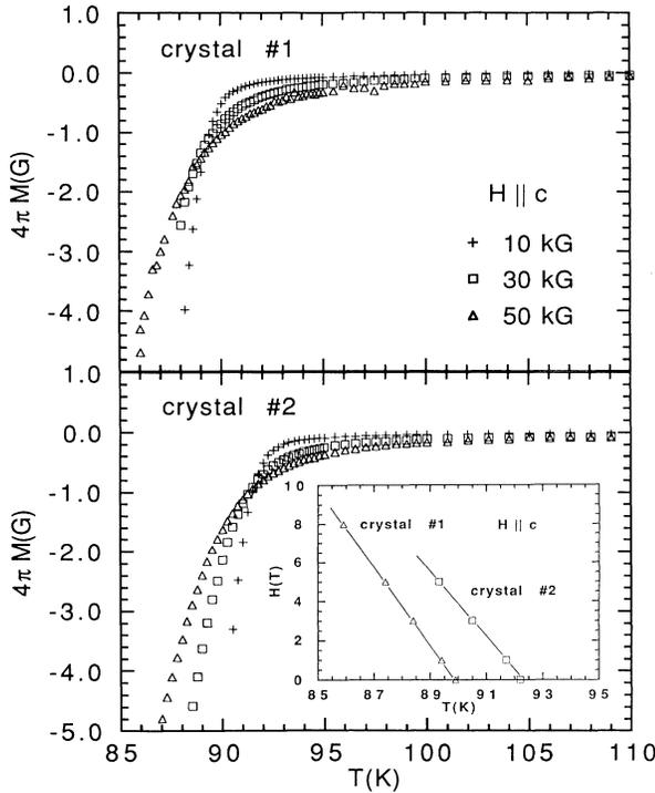
FIG. 1. Temperature dependence of the magnetization of crystals No. 1 (top) and No. 2 (bottom) in different fields parallel to **c**. Inset:  $H_{c2}(T)$  for both crystals as determined from the scaling.
