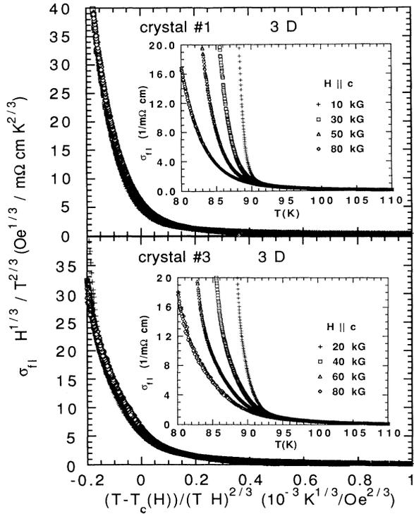
FIG. 3. 3D scaling of the fluctuation conductivity of crystals No. 1 and No. 3. Inset: The temperature dependence of the fluctuation conductivity.
