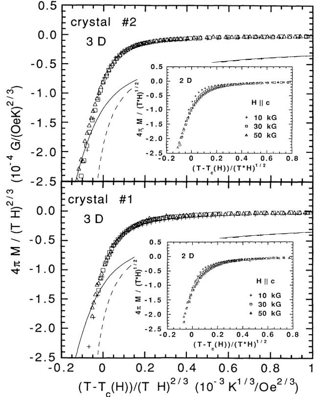
FIG. 2. 3D scaling of the magnetization for crystals No. 1 and No. 2. Insets: The 2D scaling behavior.
