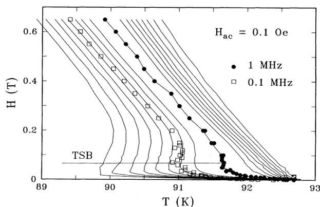
FIG. 4. Lines obtained from the maximum in  $\chi''(T, H)$  at 1 MHz (irreversibility line shown as solid dots) and 0.1 MHz (open squares). The low-field anomaly is present in both and is consistent with the thermal softening boundary (TSB)  $B \propto T^2$  [see Eq. (2)], indicated as a solid line; TSB crosses the irreversibility line. The contours probing the nonlinear regime below  $H_{irr}(T)$  also show the anomaly, suggesting a change in the pinning behavior.
