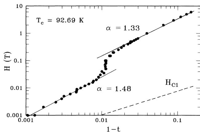
FIG. 3. Same as Fig. 2(a) for  $H_{dc}^{\parallel}$  on a log-log scale. The lines represent fits of the data by the power laws below and above the collapse edge. The high-field exponent  $\alpha$  is  $\approx \frac{4}{3}$  and at low fields  $\alpha \approx \frac{5}{2}$ .  $H_{c1}^{\parallel}$  is also shown.
