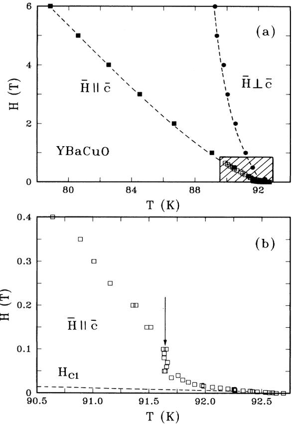
FIG. 2. (a) Irreversibility lines for the  $\text{YBaCuO}$  crystal of Fig. 1 for  $H_{dc} \perp$  and  $\parallel$  to the  $c$  axis measured at 1 MHz with  $H_{ac} = 0.1$  Oe. (b) Details of the irreversibility line at low fields for the  $H_{dc}^{\parallel}$  orientation [the shaded region in (a)].  $H_{c1}^{\parallel}$  is shown for comparison.
