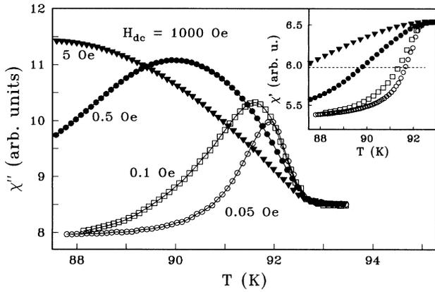
FIG. 1. Out-of-phase component of the ac susceptibility  $\chi''$  measured in a single crystal of  $\text{YBa}_2\text{Cu}_3\text{O}_7$  at 1 MHz in 1000-Oe dc field for several amplitudes of  $H_{ac}$ . Inset: Corresponding  $\chi'$  curves. Half screening is indicated by the dashed line.
